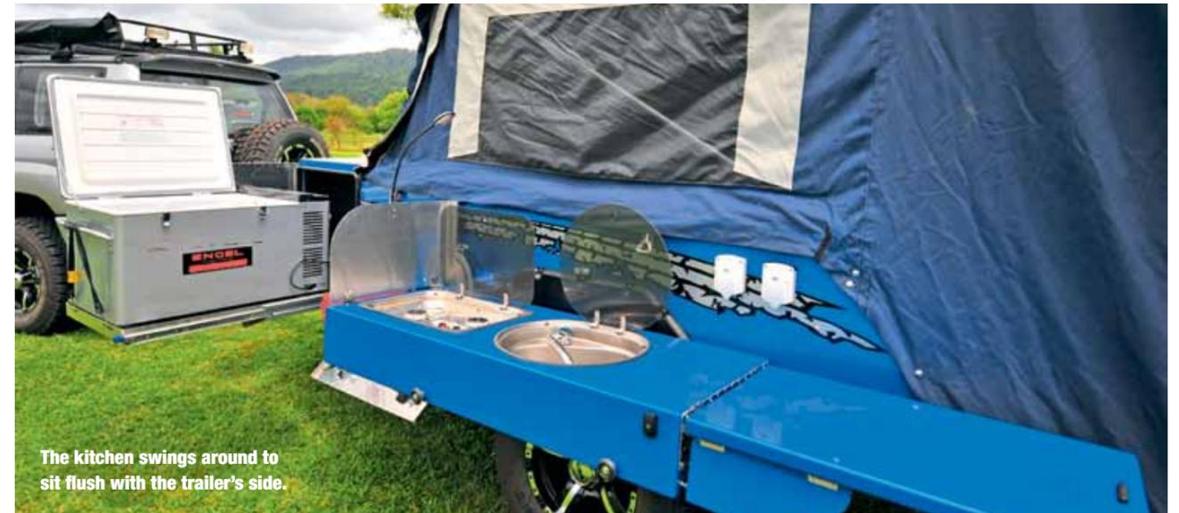
The kitchen swings around to sit flush with the trailer's side.
